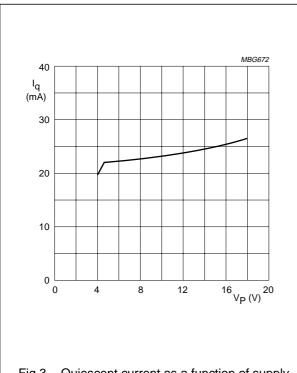
Fig.3 Quiescent current as a function of supply voltage.
