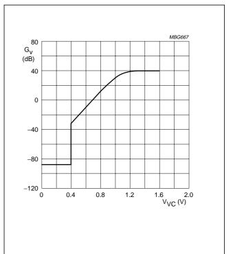
Fig.8 Voltage gain as a function of volume control voltage.
